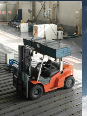
Impact test of overhead guard
