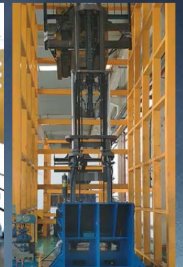
Fatigue test of lifting system
