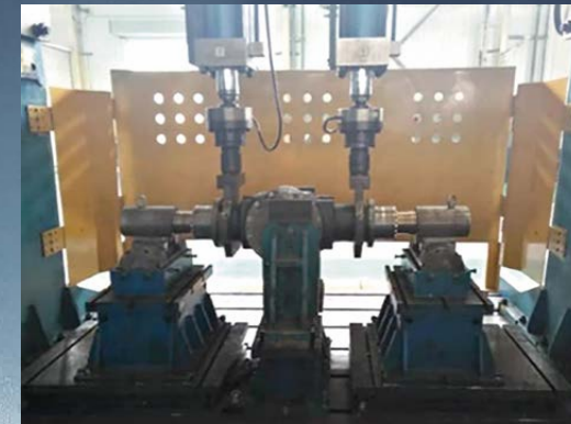
Fatigue test of drive axle
