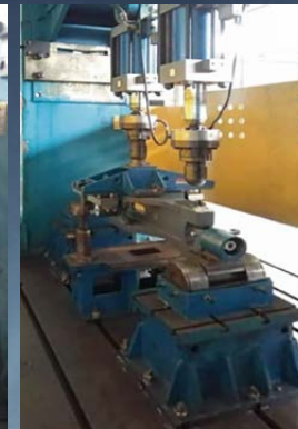
Fatigue test of steering axle
